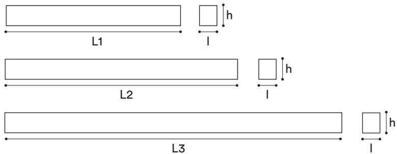
Dimensions : L1 = 600 mm, L2 = 880 mm, L3 = 1157 mm, l = 64 mm, h = 70 mm
